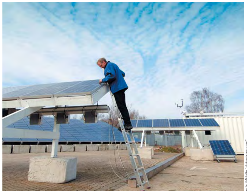
Measurements in the PHOTON laboratory: the STC-output of a module is determined by the flasher within a split second. The measurement of the yield will take a little longer – namely, one year on the free-field test facility.
