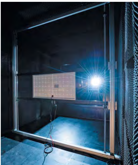
Measurements in the PHOTON laboratory: the STC-output of a module is determined by the flasher within a split second. The measurement of the yield will take a little longer – namely, one year on the free-field test facility.
